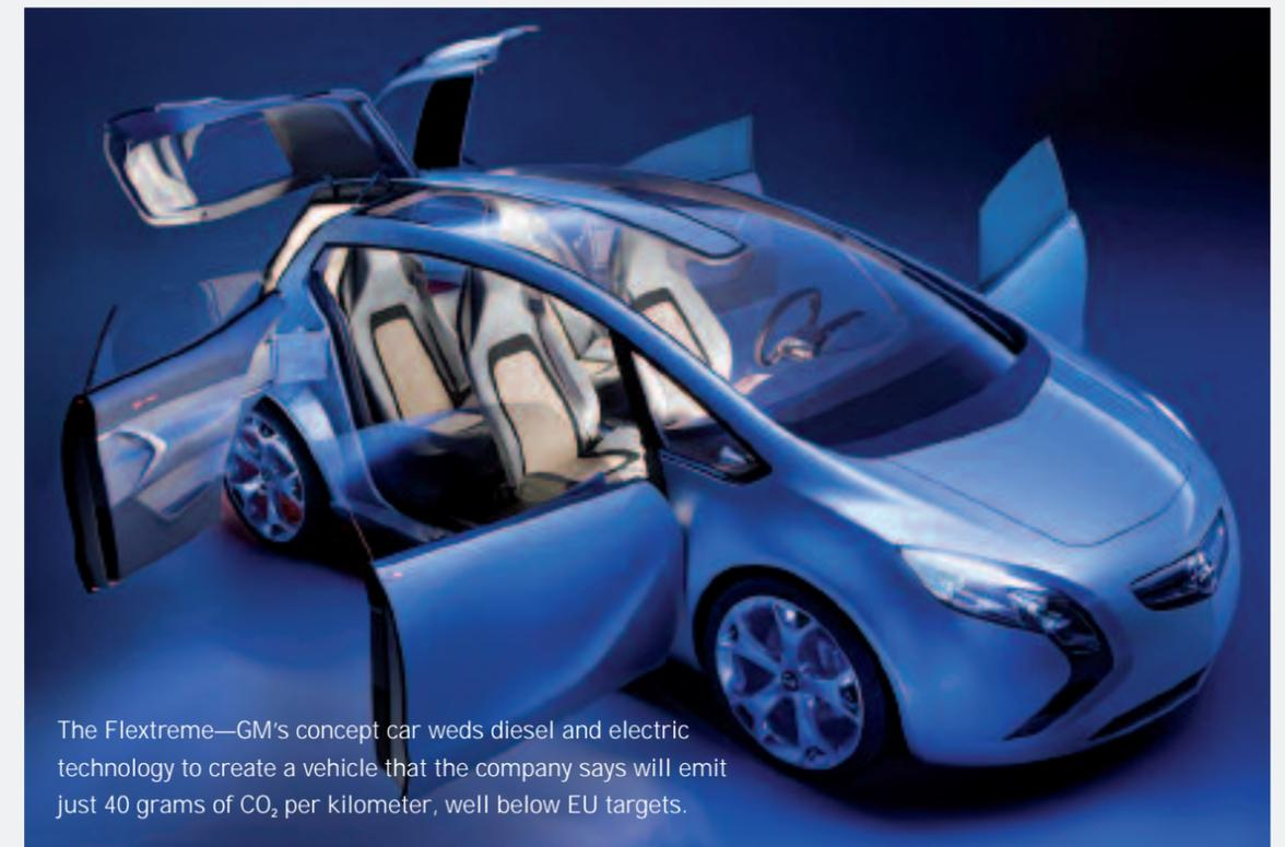
The Flextrex—GM's concept car weds diesel and electric technology to create a vehicle that the company says will emit just 40 grams of CO<sub>2</sub> per kilometer, well below EU targets.
